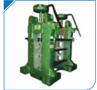
GUN METAL TYPE MILL STAND
